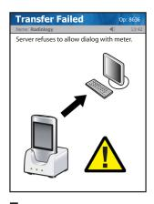
7 Server refuses to allow dialog with meter or connection to server was broken. Check network settings, network status, or contact your administrator for assistance.
