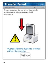
8 Meter was removed before data transfer was complete. Redock the meter.
