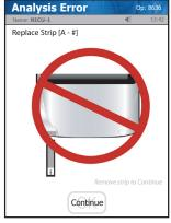
Occurs after test strip insertion or during analysis. Insert another strip and repeat the test. If the error code persists, perform the test using an alternate strip vial or alternate method.
