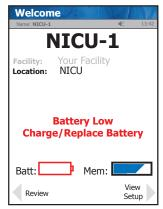
1 Change battery or place meter into charging/docking station.
