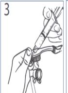
Plug center hole of feeding tube port with brush bristles. Forcefully flush moat with water.
