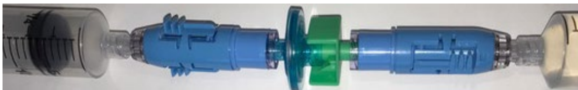
Empty Syringe - Spinning Injector - Port - Filter disc - Syringe Connector - Port - Spinning Injector - Drug-filled syringe
