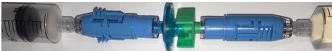
Empty Syringe - Spinning Injector - Port - Filter Connector - Syringe - Port - Spinning Injector - Drug-filled syringe
